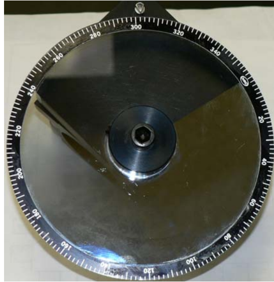
Figure 55: An image of the neutral density filter used to variably attenuate the HeNe power seen by the detector.
